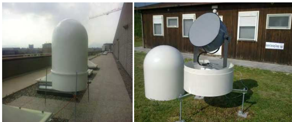
Fig. 1. The portable, low-cost weather radar with (left picture) and without (right picture) the 1-meter Diameter radome. The configuration shown here is the so-called “super-gauge”, which is a single-elevation scanning in the horizontal plane with a 3.6° beam width paraboloid (Diameter of the paraboloid is 0.6 m).
