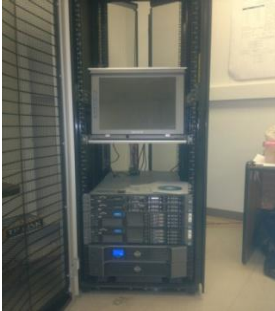
Figure 3- 1: The experimental cloud testbed based on Dell® PowerEdge® R710 and R610 Servers
