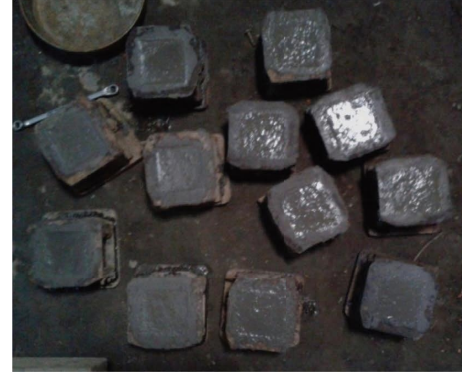
FIGURE 1: Casting of 70.6 mm \times 70.6 mm \times 70.6 mm cubic samples.
