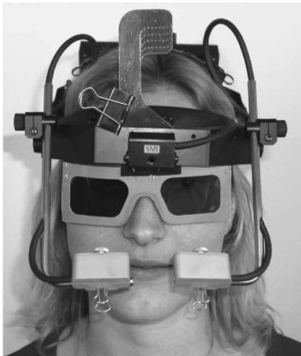
Figure 2. Eye tracker headset with 'red-green' glasses.
