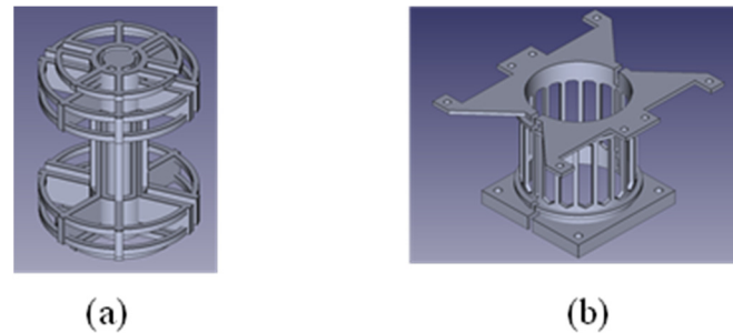
Figure 16. New support geometry for air-forced convection: (a) Inside part; (b) Outside part.
