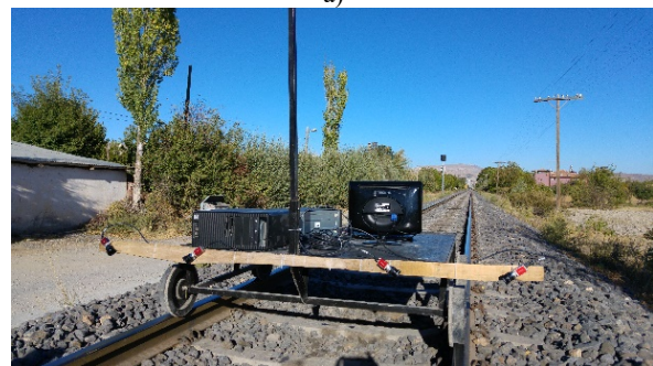
Fig. 13. Experimental design of the proposed method a) Model construction b) Installation of the test vehicle on the railway line
