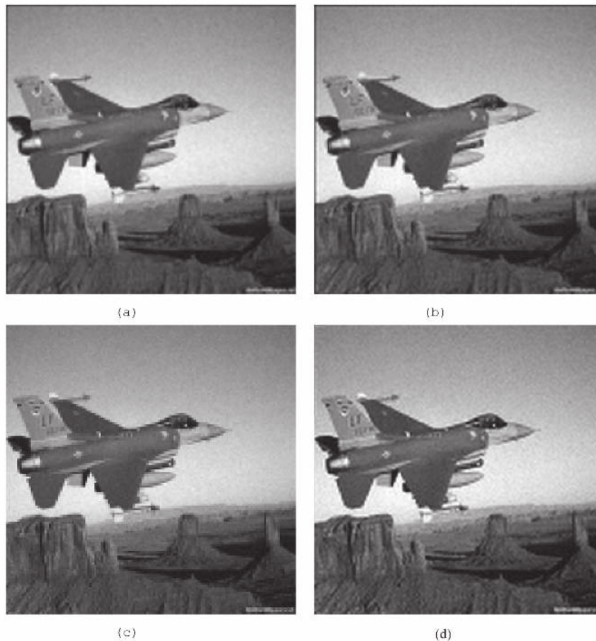
Figure 11: Interpolation Results of Plane Image. (a) Bicubic. MSE=141, a_e=0.79 . CPU= 2.6 s (b) Cubic Spline. MSE=146, a_e=0.78 . CPU=4.2 s. (c) Iterative Regularized (100 iterations). MSE=152, a_e=0.84 . CPU= 138 s. (d) Inverse Regularized. MSE=83, a_e=0.92 . CPU= 62 s
