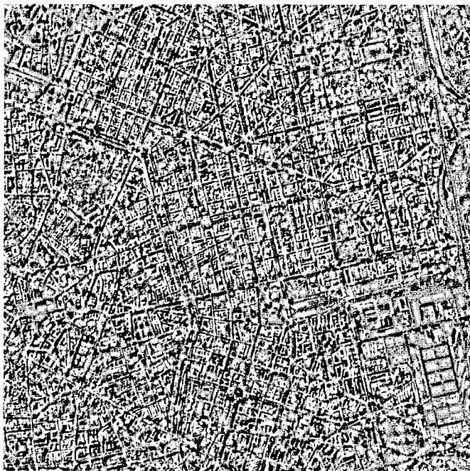
Fig. 5. Segmentation of the image in Fig. 4 by single-scale leveling (21). The utilized SE is an octagon of diameter d = 35 m (seven pixels) with \hat{k} = white, \bar{k} = black, and \tilde{k} = medium grey.
