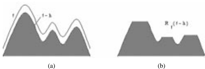
Fig. 5. (a) Example for a one-dimensional (1-D) profile (a) f and f - h . (b) Result of geodesic reconstruction. The three flatten areas show the aspect of the h maxima.
