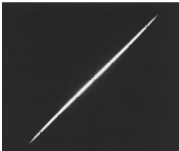
Fig. 10. Oscilloscope trace showing receiver synchronization that is maintained in the presence of modulation introduced at the transmitter. (Vertical scale: v_{C3} , 0.2 V/division; horizontal scale: v_{C2} , 0.2 V/division).
