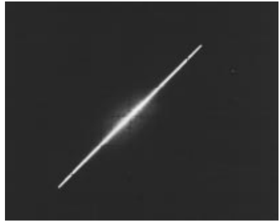
Fig. 8. Oscilloscope trace showing synchronization achieved in the first stage of the receiver shown in Fig. 5. (Vertical scale: v'_{C_3} , 0.2 V/division; horizontal scale: v'_{C_2} , 0.2 V/division).
