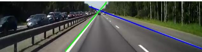
Figure 5. Left and right lane detection using Hough transform.
