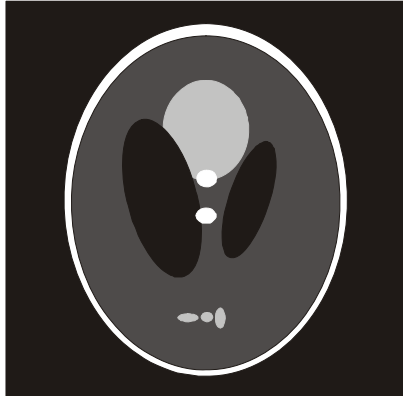
Fig. 5. A view obtained from the mathematical model of the cross-section of a skull.
