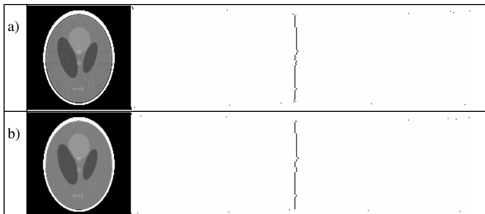
Fig. 9. View of the reconstructed image from the same projections using: (a) neural network structure, w = 6.2 \times 10^{10} , (b) convolution back-projection algorithm.
