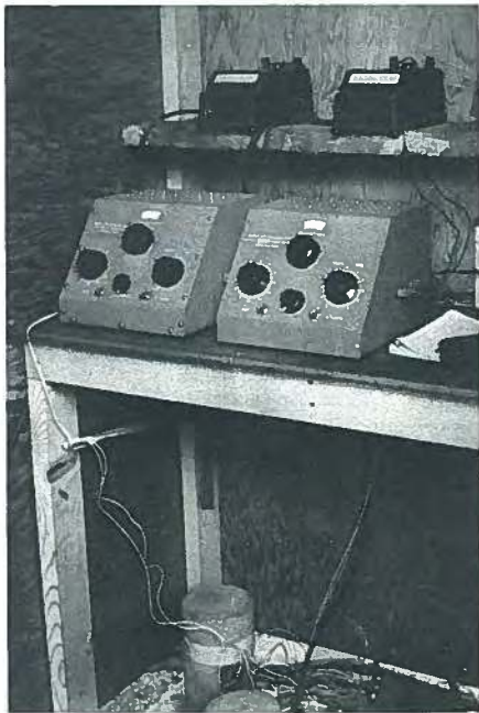
Fig. 6. Two Model 301 strainmeters used with the electric strain gages. Compensator gage is located on the test cylinder below.
