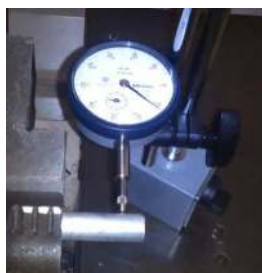
Fig. 16. Runout measurement using a dial indicator.
