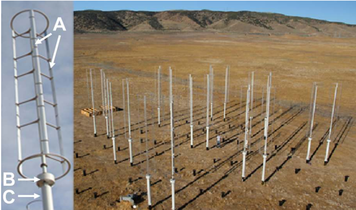
FIGURE 3. Left, Commercially-available VAWT. Vertically-oriented blades (A) with airfoil cross-sections rotate around the vertical axis of the turbine, turning an electrical generator (B) mounted on the tower (C). Right, Caltech Field Laboratory for Optimized Wind Energy (FLOWE). Arrays of up to 24 commercially-available VAWTs are tested in various configurations to study aerodynamic interactions and power generation. Scale is indicated by person standing in center of array. Video is available at http://www.youtube.com/watch?v=cZu-4Plk_5A .
