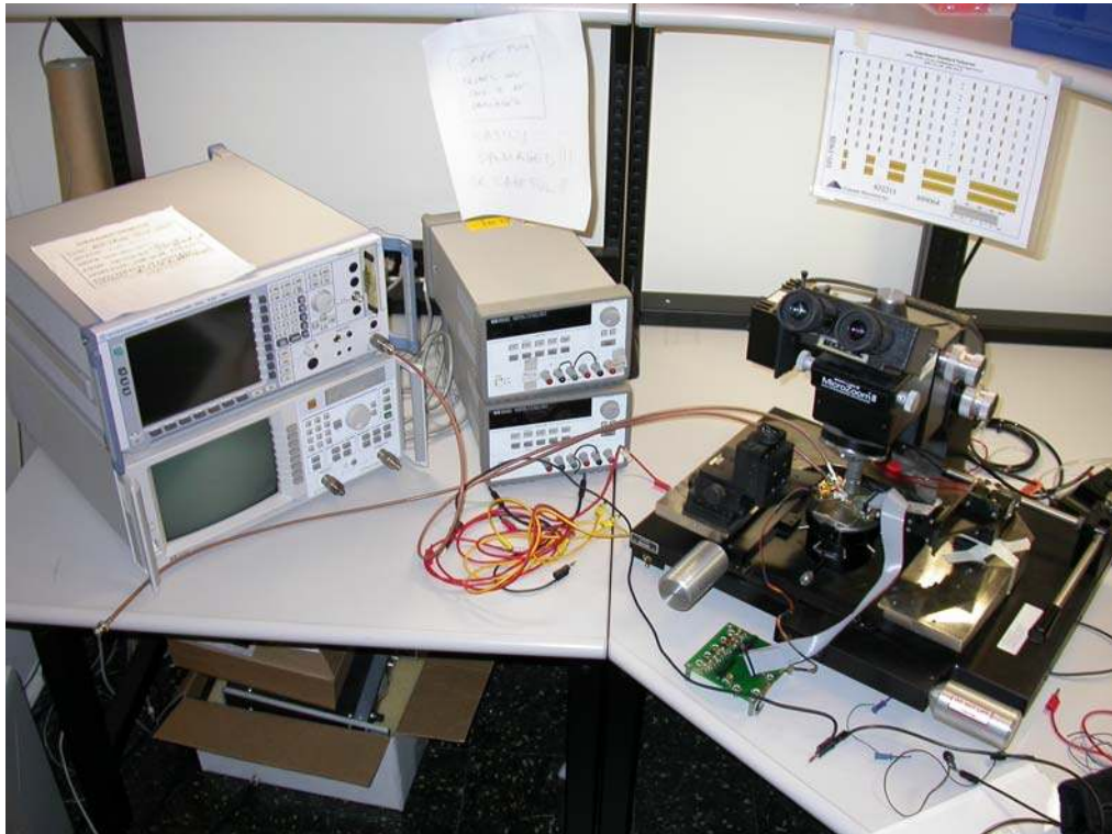
Figure 6.12 Photograph of the probing station and the test instruments.
