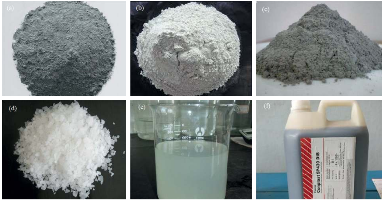
FIGURE 1: Raw constituents of the geopolymer mortar. (a) FA. (b) GGBFS. (c) Quarry dust. (d) NaOH flakes. (e) Sodium silicate solution. (f) Superplasticizer.
