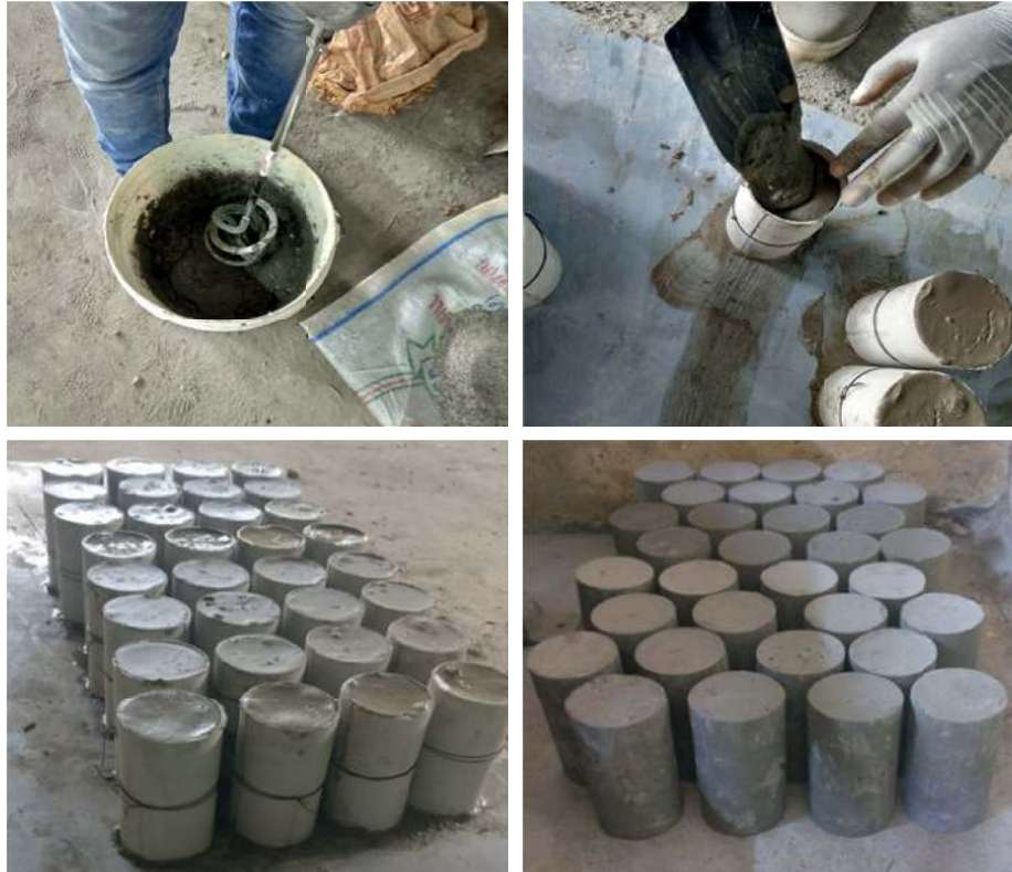
FIGURE 2: Mixing, casting, cast specimens, and demoulded geopolymer mortar specimens.
