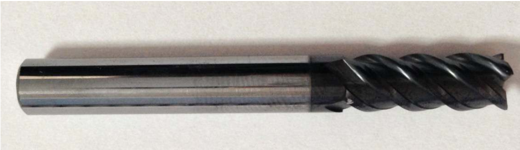
Figure 5.4 End-mill manufactured with CNC grinding machine.
