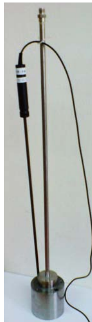
Figure 5: stainless steel cell for water vapour partial pressure measurements
