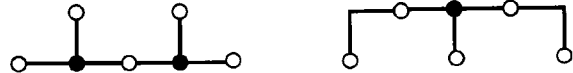
Fig. 9. A five-point example where the iterated 1-Steiner performance ratio is 7/6 . The optimal MRST (left) has cost 6, while the (possible) heuristic output (right) has cost 7.
