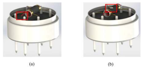
FIGURE 12. The structure of HWD fault and ESB fault (a) HWD fault and (b) ESB fault.
