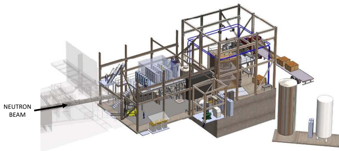
Figure 4. General layout of the nEDM apparatus and associated infrastructure at the SNS. External magnetic field coils are also shown outside of the Magnetic Shield Enclosure (MSE) to reduce the ambient Earth's magnetic field.
