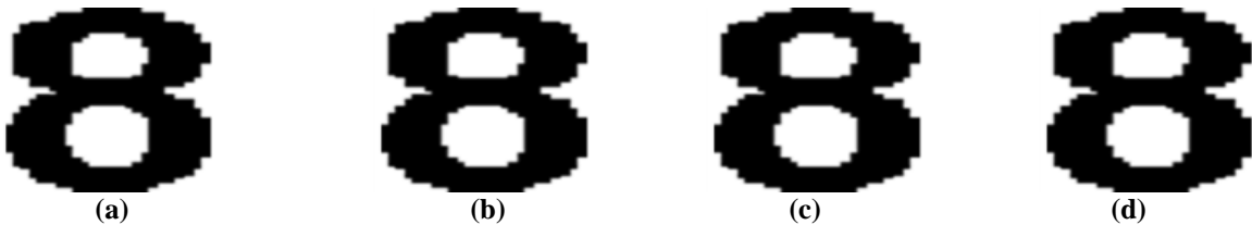
Fig.7 (a) Original Watermark (b) Watermark extracted from 1 st frame of News.y4m video (c) Original Watermark (d) Watermark extracted from 48 th frame of News.y4m video
