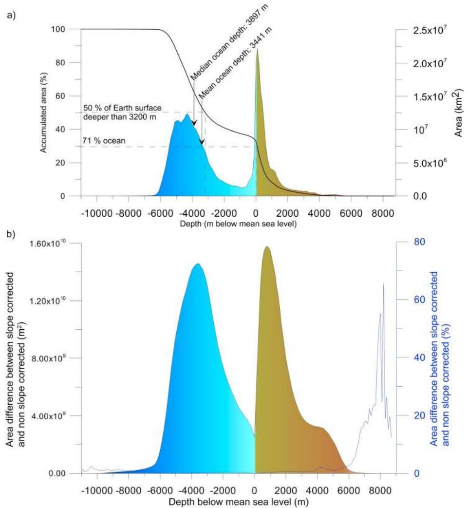
**Figure 8.** Earth’s hypsometry from GEBCO\_2014. (a) The filled curves are the distribution of ocean depths (blue) and land elevations (brown) relative to calculated area (right y axis); the solid black line is the accumulated area in percent (left y axis). (b) Comparison between slope-corrected and nonslope-corrected hypsometric calculations, the colors are the same as in Figure 8a.
