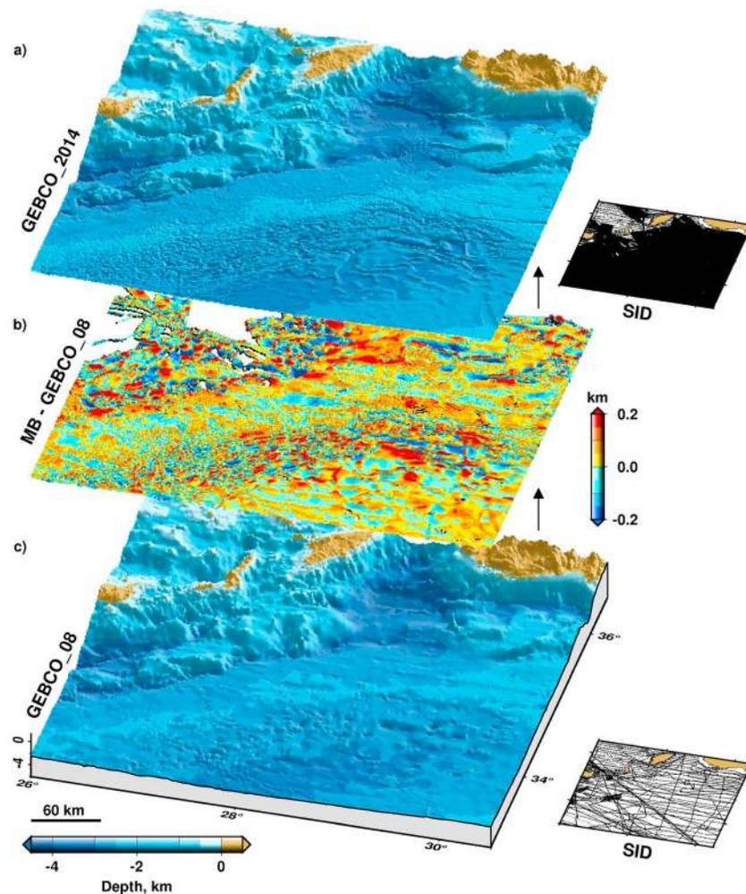
**Figure 4.** Example of how multibeam data are ingested into the GEBCO\_2014 grid using the remove-restore procedure. The (b) differences between GEBCO\_08 and multibeam data are added to (c) GEBCO\_08 to form the (a) new GEBCO\_2014 grid. SID maps demonstrate the improved sounding coverage.
