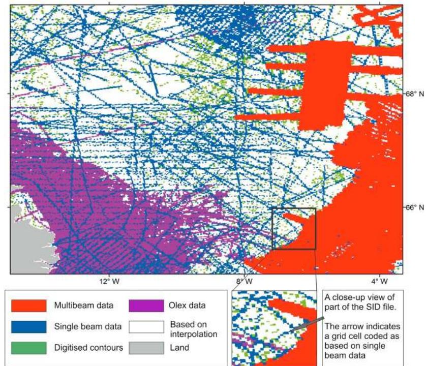
**Figure 3.** Image based on the Source Identifier (SID) grid (enlarged area from Figure 2). The SID grid can be used to identify the source data used to generate the GEBCO\_2014 grid for individual grid cells.
