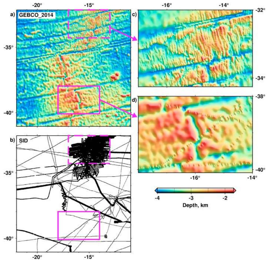
**Figure 7.** (a) GEBCO\_2014 bathymetry model over the southern Mid-Atlantic Ridge and (b) locations of depth constraints used in model. North-south trending abyssal hills flanking the spreading ridge axis are resolved in Figure 7a (dashed box) and enlargement (c) because multibeam data were incorporated into the bathymetry model. (d) Abyssal hill fabric is only hinted at where depths are estimated primarily from satellite altimetry.
