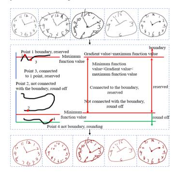
Figure 3. Contour edge detection process
