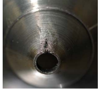
(b) Picture of the magnetron puller electrode after a few days of testing. The traces originate from the deviated electron beam and the outer parts of the H^- beam.
