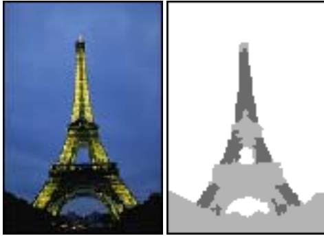
Figure 7. A 121 \times 82 color image (left) and its segmentation (right). Parameter settings: \sigma = 0.325 . Minimal region size of interest is 10.
