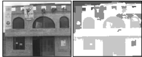
Figure 5. A 94 \times 115 intensity image (left) and its segmentation (right). Parameter setting: \sigma = 0.15 . Minimal region size of interest is 11.
