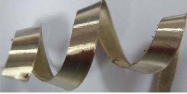
Fig. 5 Experimental chip morphology: continuous chip without segmentation
