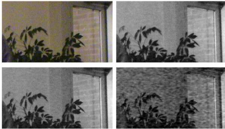
Figure 1. Portion of an image captured with a Sony DCR-TRV27; and its red, green, and blue channels. The blue channel is the most degraded channel. The noise apparently has coarse-grain and fine-grain components.
