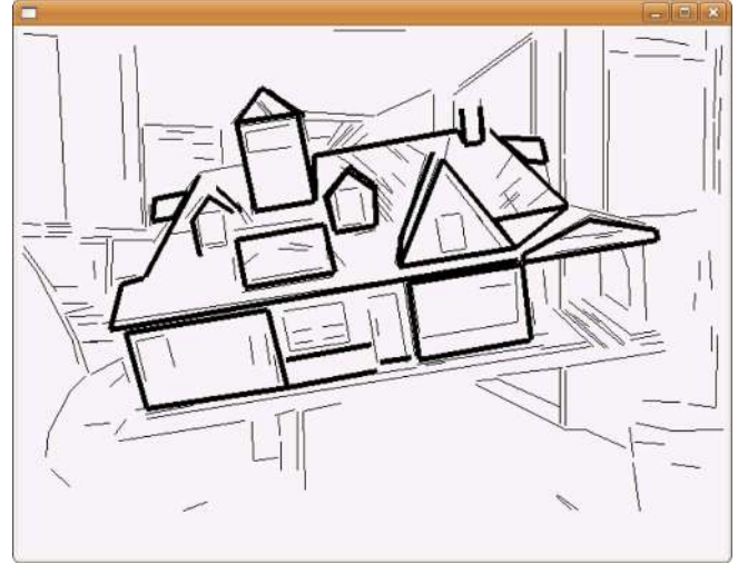
Fig. 4. For the pose of the object shown, the expectation map as derived from the 3-D object model consists of the thick black lines in the figure. The thin black lines shown in the figure constitute the scene features extracted from the image.
