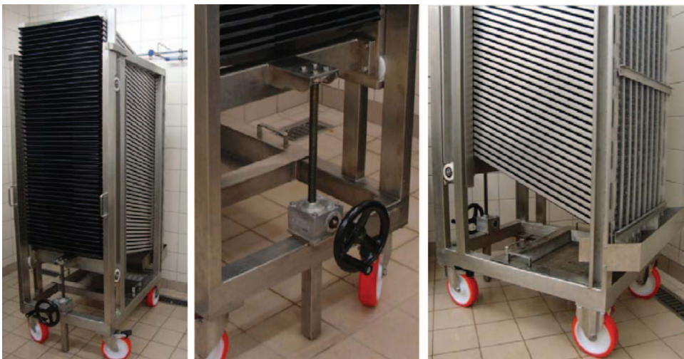
Fig. 2. Rack unit. (Left) Front view of the rack structure fully stacked with trays in tilted position. (Center) Detail of the endless screw jack system and its hand wheel controller. (Right) Back view of the bottom frame of the rack with the plastic curtain, the metallic slide and the basket collector. (Online figure in color.)
