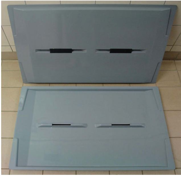
Fig. 1. Mass rearing tray. The ridges which create the overflow system and increase larval resting space availability are visible on the lower tray. The underside of the tray shows the two plastic plates which deflect the overflowing water to avoid water falling straight down. (Online figure in color.)
