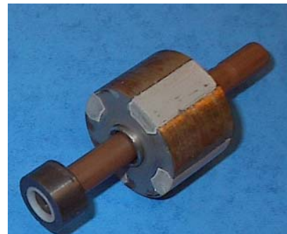
Fig. 7 A picture of the rotor of the prototype HSR motor
