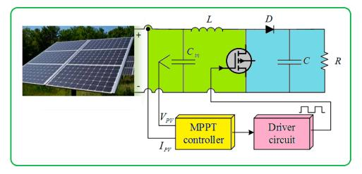
Figure 4. Block diagram of an ROA-based MPPT.
