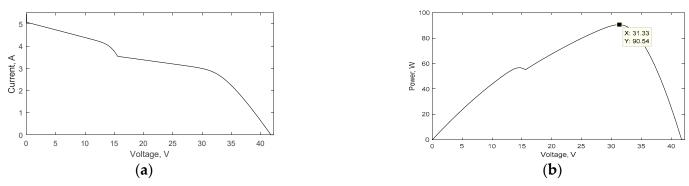
Figure 7. Characteristics of PV panel for pattern 2: (a) P-V, (b) I-V.
