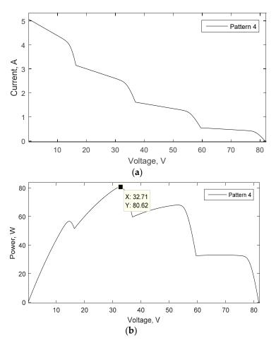
Figure 14. Characteristics of the PV panel for pattern 4: (a) P-V, (b) I-V.
