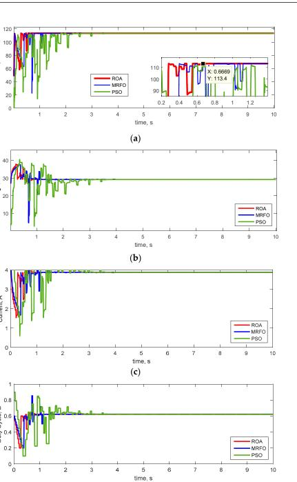
**Figure 9.** (a) PV power, (b) PV voltage, (c) PV current, (d) Duty cycle in pattern 1 using different methods.
