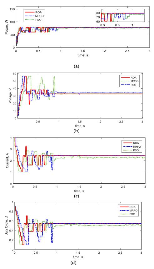
Figure 15. (a) PV power, (b) PV voltage, (c) PV current, (d) Duty cycle in pattern 4 using different methods.
