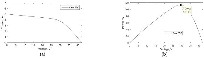
**Figure 6.** Characteristics of PV panel for pattern 1: (**a**) P-V, (**b**) I-V.
