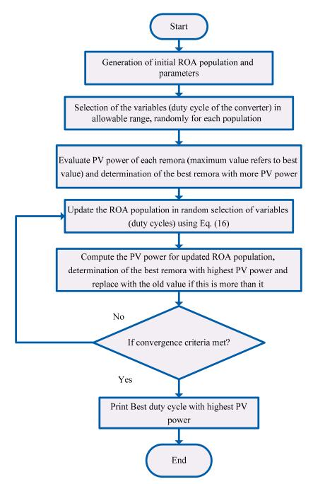
Figure 5. Flow chart of ROA implementation in proposed MPPT solutions.
