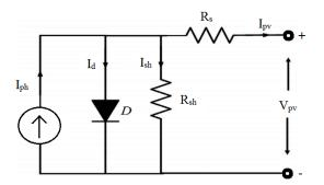
Figure 1. PV Model as single-diode.
