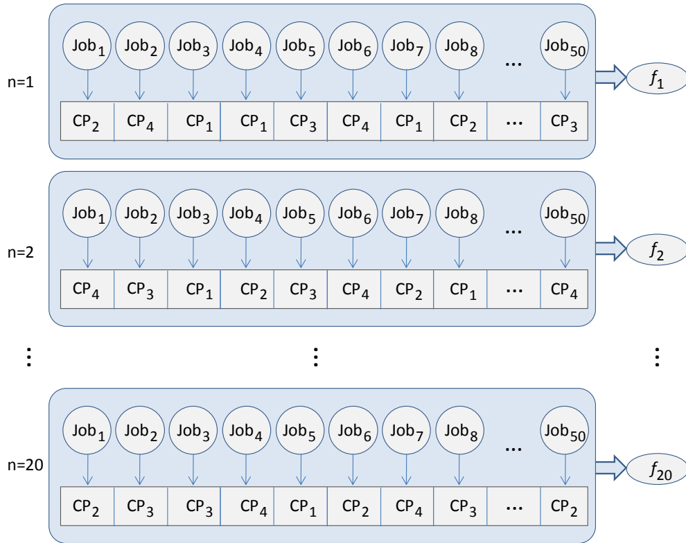
Figure 4-13 An example for proposed GA-based job-scheduler to distribute jobs from Cloud Subscriber to 4 other Cloud Providers. It is assumed that number of jobs for each step is x=50 , the iteration number is n=20 , the crossover-rate is 0.1 and the mutation-rate is 0.02.
