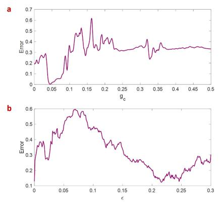
**Figure 4.** Synchronization error of the network of 100 memristive neuron maps connected through (a) chemical and (b) electrical synapses by the variation of coupling strengths. The network parameters are  $\Theta_s = -40$ ,  $\beta = 50$ , and  $v_s^* = -40$ . Complete synchronization can be observed in chemically coupled neurons for  $0.0427 \le g_c \le 0.0463$ .
