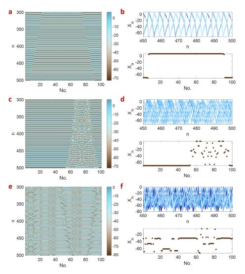
**Figure 7.** The spatiotemporal patterns (left panel) and the time series and snapshots (right panel) of the network of 100 memristive neuron maps coupled via electrochemical synapses. (**a**,**b**) For  $g_c = 0.07$  and  $\epsilon = 0.01$ , imperfect synchronization is formed. (**c**,**d**) For  $g_c = 0.05$  and  $\epsilon = 0.05$ , the chimera state is observed. (**e**,**f**) For  $g_c = 0.52$  and  $\epsilon = 0.11$ , the nonstationary chimera appears.
