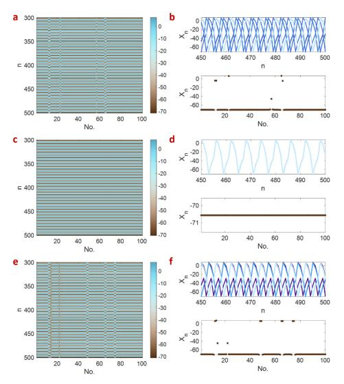
**Figure 6.** The spatiotemporal patterns (left panel) and the time series and snapshots (right panel) of the network of 100 memristive neuron maps coupled via chemical synapses. (**a**,**b**) For  $g_c = 0.04$ , imperfect synchronization is observed. (**c**,**d**) For  $g_c = 0.044$ , complete synchronization is achieved. (**e**,**f**) For  $g_c = 0.06$ , the solitary state appears.
