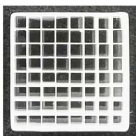
Figure 2. Image of the prototype scintillator array produced by CPI Inc.
