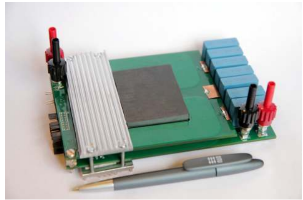
Fig. 15. Parallel primary 1600W prototype, achieving a power density of 51 W/inch 3 .
