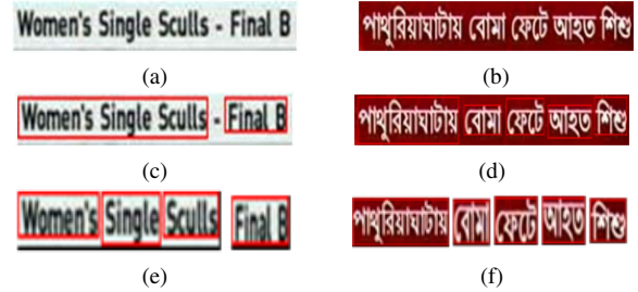
Fig. 13: (a),(b)Samples of horizontal text lines; (c),(d)Word segmentation results obtained in stage-1; and (e),(f)Final word segmentation results obtained in stage-2.
