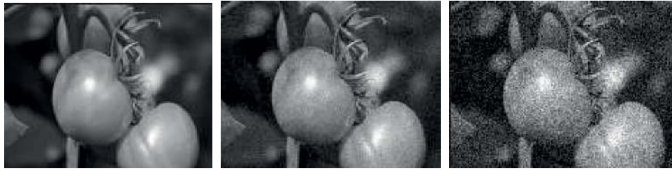
FIGURE 5: (a) Original image, (b) Gaussian noise graph, and (c) salt and pepper noise graph.
