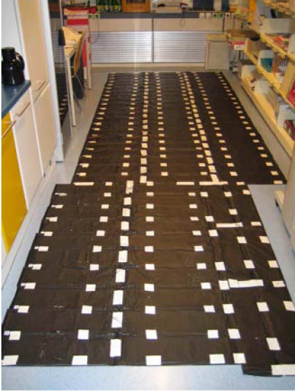
Fig. 11. Tactile floor sensors in Smart Environment.
