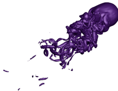
Figure 26. Vortex structure of the flow past a sphere at Re = 1000 .
