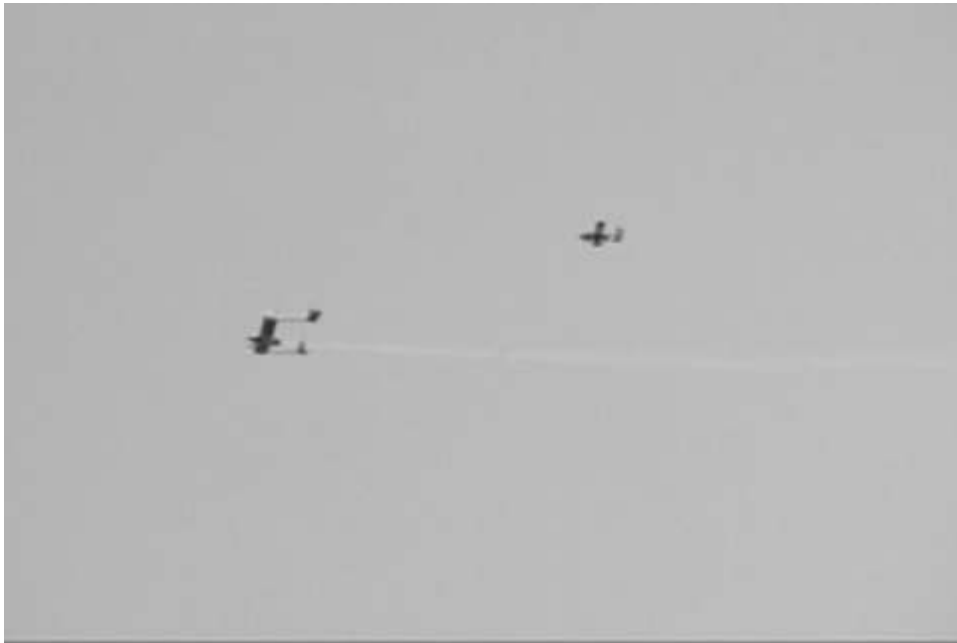
Figure 16. Formation Flight during Flight Test (The Mini is commanded 12 meters behind and 2 meters above the Parent)
