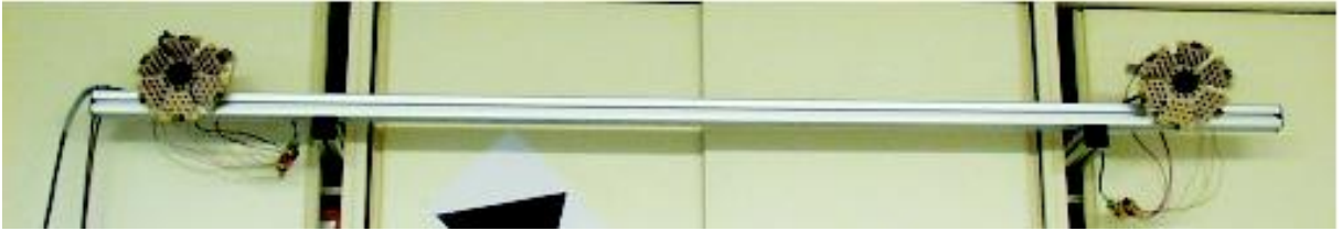
Fig. 1. Stereo rig with adjustable baseline up to 2 m, progressive scan cameras for synchronous stereo grabbing at 30 Hz, IR lighting, and IR filters.
