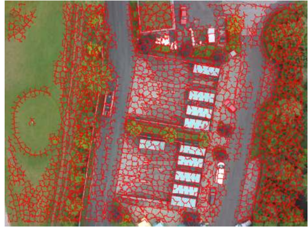
Figure 3: Feature points (red) defined as the border pixels of a superpixel segmentation step.
