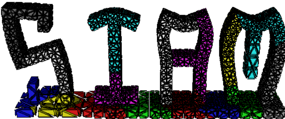
FIG. 13. An adapted mesh and solution (as a deformation), illustrating the adaptivity pattern generated by a normal global (sequential, conforming) approach on a single processor for comparison.
