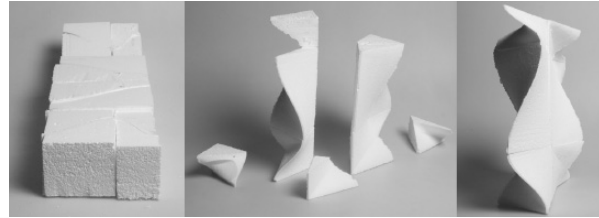
Figure 8. StackIt: A freeform wall resulting from 2x4 parametric toolpaths; cut stockmodel (left), 12 geometric entities (middle), mounted result (right). Design by Christoph Müller and Christian Vladikov.
