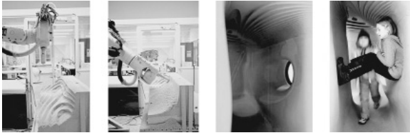
Figure 1. Robot milling for freeform surface design at TU Vienna: a 1:1 prototype is rough-cut (left), fine-cut (middle-left), finished surface (Polyurethane) (middle-right), in use (right).
