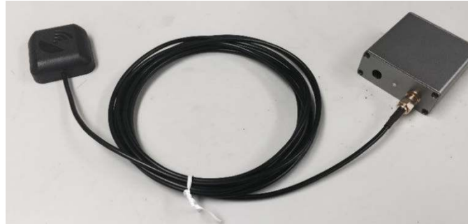
385 Fig. 9 u-blox NEO M8T GNSS module with antenna.
