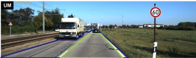
Fig. 3: Example polygonal annotation of road area (blue) and ego-lane (green) in an image from the UM dataset.
