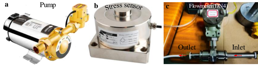
(a) Self-priming pump of LS-0412 (b) Stress sensor (c) Flow sensor of DN4 Figure 3 Monitoring components for the testing platform system
