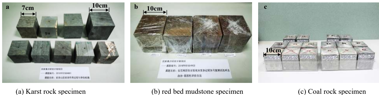
Figure 5 Standard preparations of rock specimens of different lithology
