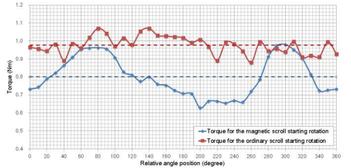
Fig. 7 Experimental results for the torques for starting rotations of the ordinary scroll air motor and the prototype magnetic scroll air motor
