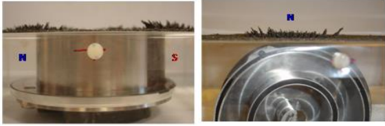
Fig. 5. Illustration of the manufactured prototype magnetic scroll air motor (N: North Pole; S: South Pole) [19]
